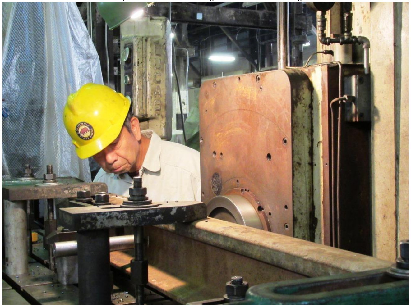
Toby monitors the big Lucas milling machine as it cuts away on the rail
